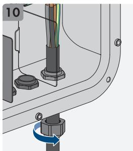
**11**  $\Rightarrow$   $PE_{AC} < 10 \text{ mm}^2$  / **Optional**  $\Rightarrow$   $PE_{AC} 10 \text{ to } 16 \text{ mm}^2$
